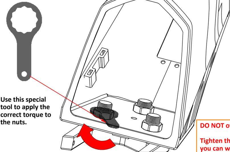
**DO NOT over tighten the screw.**
