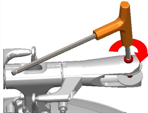
**3** Check main hub screws(M4x24 and 2 M3x12) Ensure they are tight.
