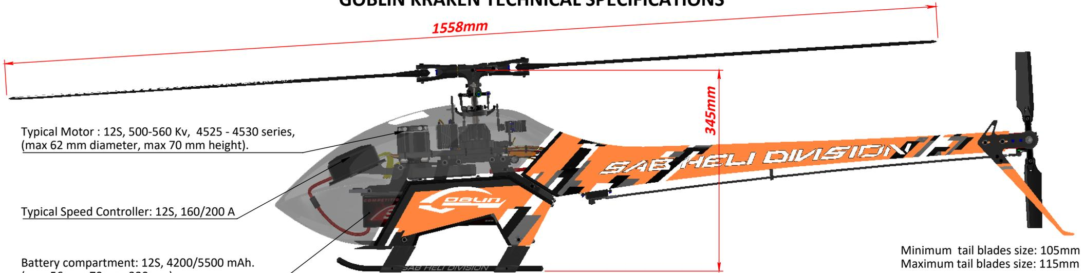
Typical Motor : 12S, 500-560 Kv, 4525 - 4530 series,
