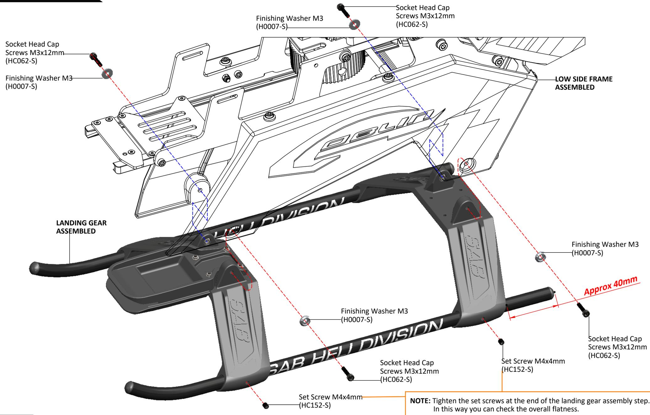
**NOTE:** Tighten the set screws at the end of the landing gear assembly step. In this way you can check the overall flatness.
