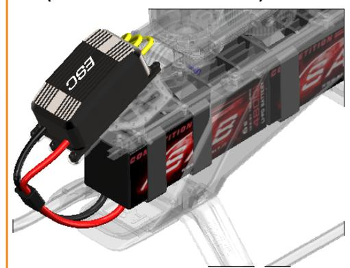
**5** Check Tail & Motor belt tension. The tension has to be tight.
